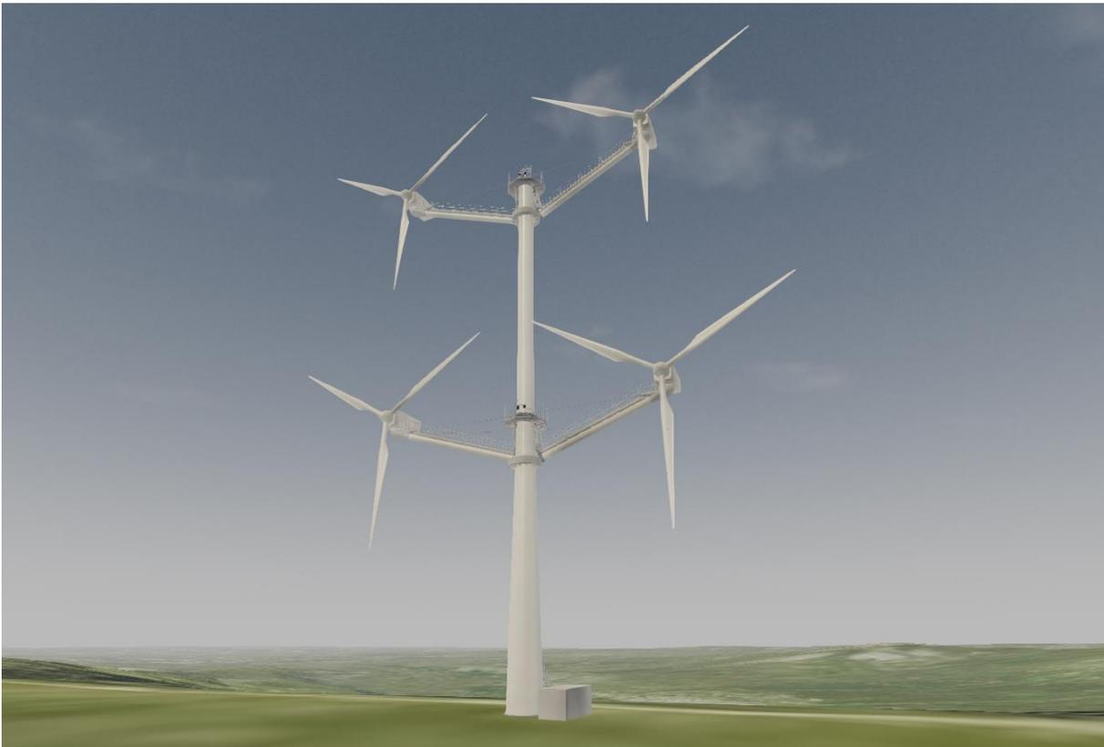
(Illustration of the multi-rotor concept demonstration turbine)
