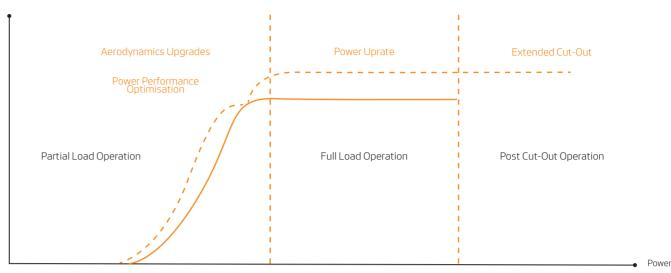
Display of the PowerPlus solutions and their impact on AEP on the different stages of the power curve
