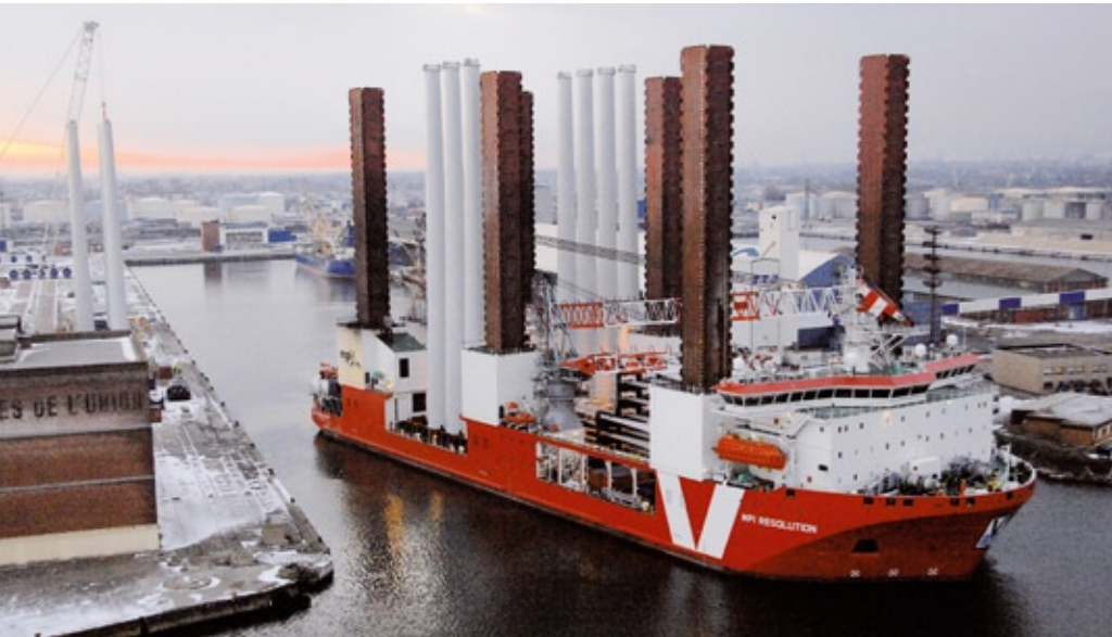
◀ The 'MPI Resolution' transport vessel with Vestas turbines on her way to the offshore installation at the Thanet wind farm
