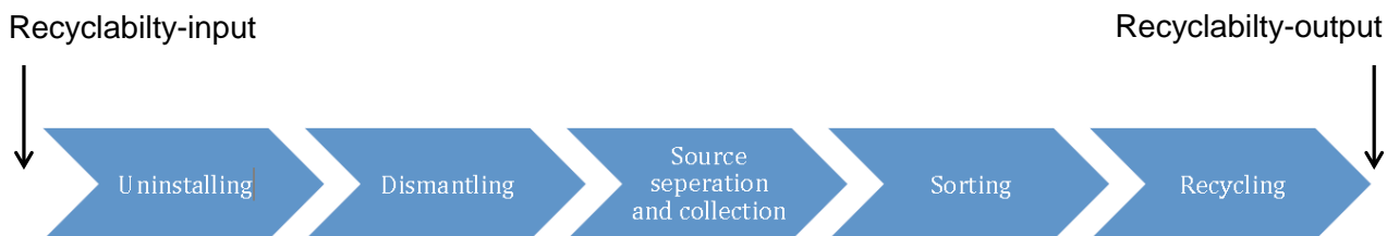
Figure H2: Recyclability-input and Recyclability-output of the wind turbine
